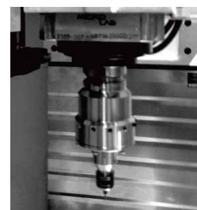
Ultrasound spindle to cut honeycomb plate (opt.)
